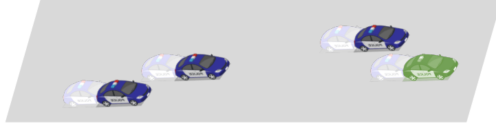
Figure 3.4: All vehicles in the segment (blue) are considered to be following a virtual vehicle (green). If the car-following is exact, the separation (distance) between each vehicle is maintained, which is also the optimal scenario.
